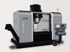
Our 5-axis CNC machining centers, equipped with the integrated Hurco control, are simply the best in the industry. Our control simplifies the transition from conventional 3-axis to 5-axis machining. Our 5-axis mills are the only ones that have UltiMotion, our patented motion system that cuts cycle time by up to 30% while increasing the quality of the part's surface finish.
